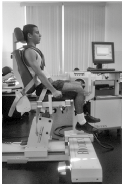
Figure 2. Volunteer positioned to the knee test on the isokinetic dynamometer Biodex® Source: prepared by the authors.
